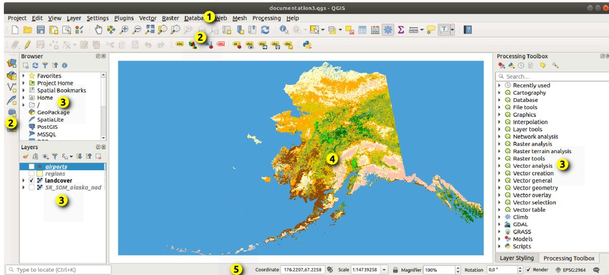
Figure 1. QGIS Graphical User Interface, showing (1) menu bar, (2) toolbars, (3) panels, (4) map view and (5) status bar. Adapted from the QGIS manual (3.28).
